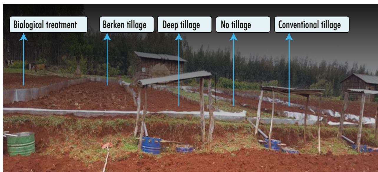
Figure 18: Sets of experiments on how different depth of tillage and breaking of the hard pan affects soil penetration resistance, infiltration, runoff, erosion and biomass yield.
