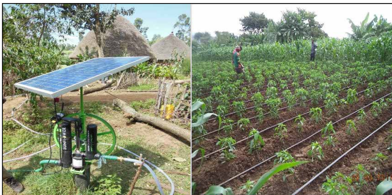
Figure 24: Solar pump linked to drip system in central rift valley (Photo credit: Amare Hailelassie).
